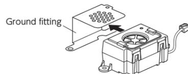
2. Pull the 4 hooks on the lower case outwards, and remove the upper case. Remove the 2 screws, and remove the buzzer from the lower case. [See Fig. 1]
